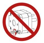
Use the extended screws for mounting but do not adjust them. Take normal vacuum precautions, avoid creating trapped volumes when mounting the motor and obstruct as few as possible of the pumping holes in the end faces. The location spigot projecting from the face of the motor is accurately concentric with the shaft and intended for precise location in a recess.
