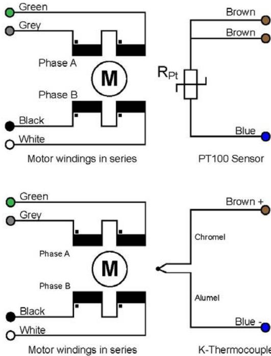
If the identification beads have been removed then use the following procedure. An ohmmeter with resolution down to about 1 ohm is required to identify the two phase windings: most inexpensive multimeters are suitable.
