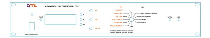
Turn the rotary switch to the 'Off' position.
