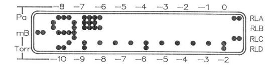
The entire display can be replaced by a display of the gauge assignment and trip pressures of the relays, by pressing the "Trip" switch. More information on this is contained in section 3:5.2, below. Pressing the "Trip" switch a further four times will restore the former display.
