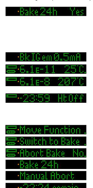
Start Bake by turning the Function Switch to BAKE and press ENT.
