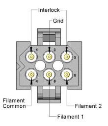
Base connections of AIG1x gauges.
