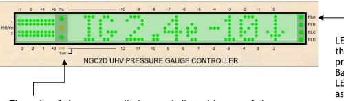
The units of the pressure display are indicated by one of three LEDs in the display area. The centre orange LED indicates that mBar has been selected, the green LED above it indicates Pascal and the green LED below indicates Torr.
