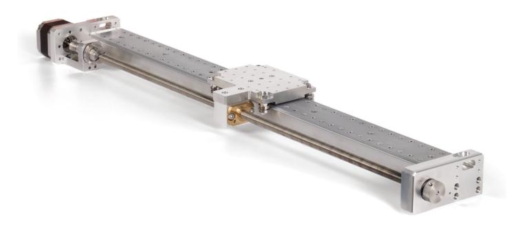
Extra long travel ultra-high vacuum compatible modular linear translation stages provide long travel with minimum height for loads of up to 20 kilograms. They have widely spaced 'V' roller guides and are useful in in applications where extra long travel is required but torsional loads are small.
