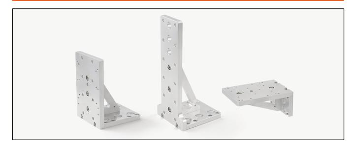
AML UHV compatible mounting brackets for use with VSM stages. Used to reorient stages or design multi-axis mechanism with standard products. AML mounting brackets are constructed with lightweight uhv-prepared aluminium to reduce mass whilst maintaining stability.
