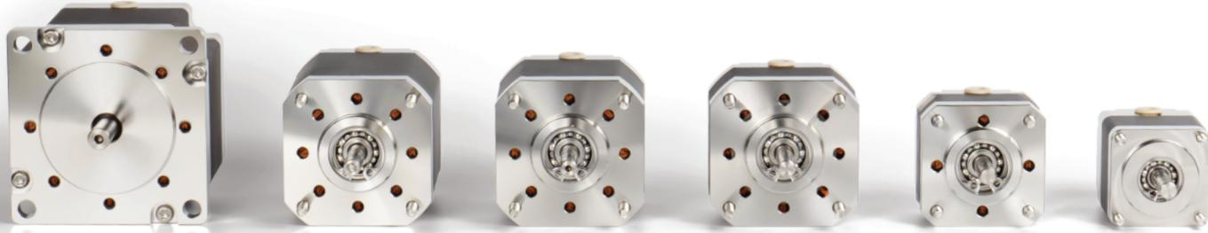
The model D motors are two phase hybrid stepper motors, available in a range of standard sizes and torque ratings. Standard motors provide 200 full steps per revolution, are suitable for use below  $1 \times 10^{-10}$  mbar and working temperatures between -65 °C to +190 °C. Extended low temperature range (-196 °C) versions, radiation hard versions ( $1 \times 10^6$  Gy), shaft modifications and hybrid bearings are all available options.
