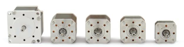
The model D motors are two phase hybrid stepper motors, available in a range of standard sizes and torque ratings. Standard motors provide 200 full steps per revolution, are suitable for use below  $1 \times 10^{-10}$  mbar and working temperatures between -65 °C to +190 °C. Extended low temperature range (-196 °C) versions, radiation hard versions (1 x  $10^6$  Gy), shaft modifications and hybrid bearings are all available options.
