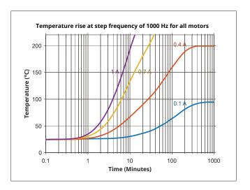
Use of the embedded temperature sensor is essential for motor protection. Irreversible damage of the motor windings will occur if the temperature exceeds the stated maximum operating temperature.
