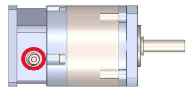
2. Position the motor vertically with the shaft pointing upwards and insert the motor shaft into the gearhead shaft clamp.
