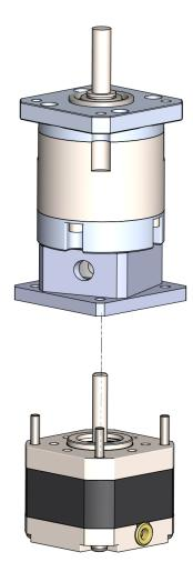
3. Once the gearhead is fully seated, secure with the  $4 \times M3$  nuts supplied. Recommended torque  $\sim$ 1.4Nm (12.39 in-lbs).
