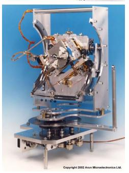
Stepper motor-based mechanisms should not be regarded merely as replacements for those based on other techniques, since they offer specific advantages and are suitable for applications not addressable by other means. The advantages of internally motorised mechanisms are that the number and range of motions, rigidity, accuracy, repeatability, speed, reliability and crosstalk between motions are much better than is possible
