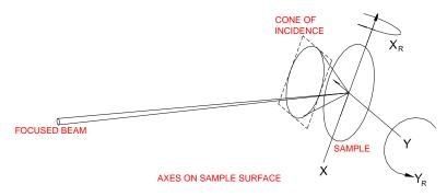
Using vacuum motors the XY axes are fixed on the sample surface and the rotation axes are Therefore, if the same. incidence angle of changed the point of incidence does not change. The incidence
